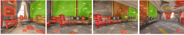
Fig. 8. Successful navigation example in Habitat using continuous control mode to reach the green painting goal in the rightmost image. The horizontal pixel offset (depicted through the length and direction of arrow) for each of the matched query segments is weighted by the path length to the goal (depicted through color with length decreasing from red to green), to generate an aggregated angular velocity.
