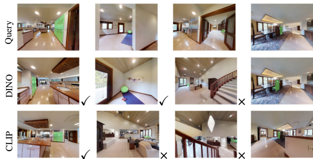
Fig. 4. Object Instance Recognition in GibsonEnv [63]: The rows show segment masks (in green) for the query, DINO match, and CLIP match respectively. Symbols (✓/×) adjacent to images indicate success or failure in association. The final column illustrates category-level recognition success despite both methods failing at the instance level (multiple chairs in close proximity).
