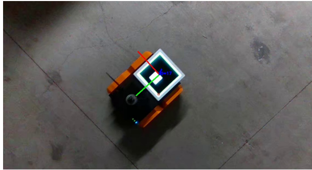
Fig. 5: Looking down ↓ Robot Detection from Environment Camera: The Calibration Robot (Figure 4) viewed from an environment camera with axes drawn on the detected backlit ArUco marker.
